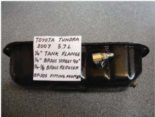
TANK FLANGE ON THE SIDE OF THE OIL PAN.
