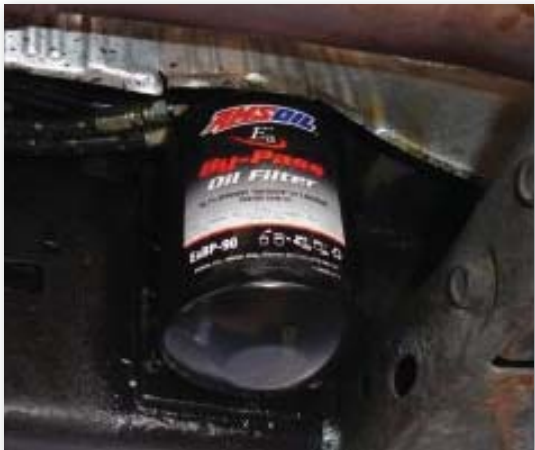
AN 8" x 4 1/2" x 3/8" MOUNTING PLATE HOLDS THE FILTRATION SYSTEM.
