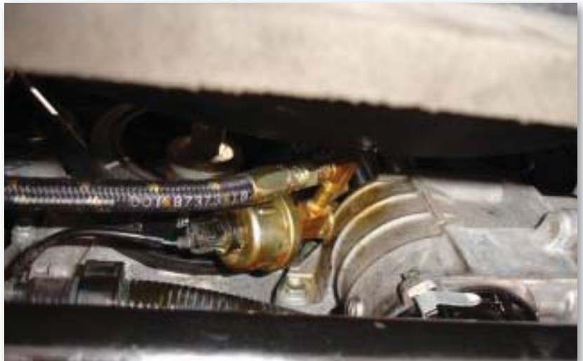
SUPPLY LINE TO OIL SENDING UNIT.
