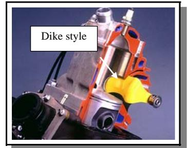
The movement of the valve can be controlled in several differing ways. Some designs use exhaust or cylinder pressure to activate the valve while others use an electro/mechanical method. A third style uses a direct cable or mechanical linkage to operate the valve. Though each design has its own benefits and disadvantages, all suffer from a similar problem. That problem, is that they all require periodic maintenance.
