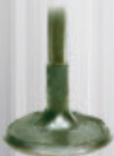
Intake valve after P.i. treatment
