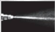
Injector spray pattern before P.i. treatment
