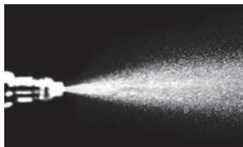
Injector spray pattern after P.i. treatment.
