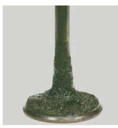
Picture D - Intake valve before P.i. treatment
