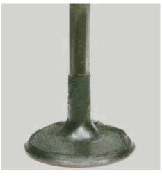
Picture E - Intake valve after P.i. treatment
